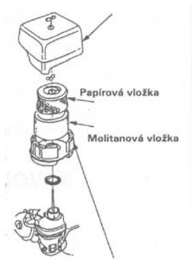
**Fig. 2 Air filter - HATZ engines**
